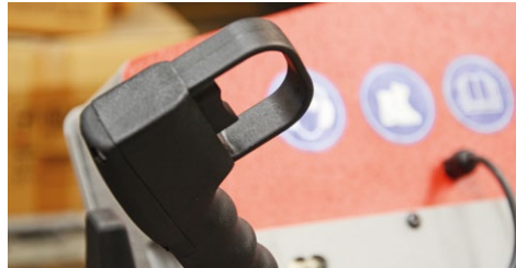
Ergonomic handle for starting the saw band and the arm's cutting
