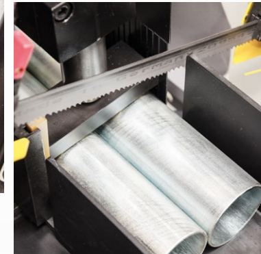
Automatic downfeed pressure regulation
