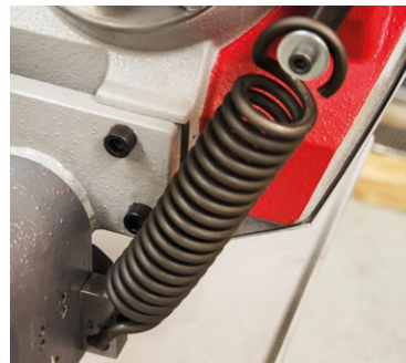
Flexible spring for easy movement of the arm to the cut and returning back to the top position
