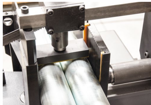
Automatic downfeed pressure regulation
