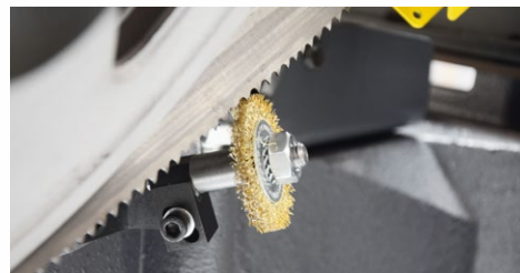
A chip brush is always driven concurrently with the speed of saw blade in order to provide an ideal cleaning effect.
