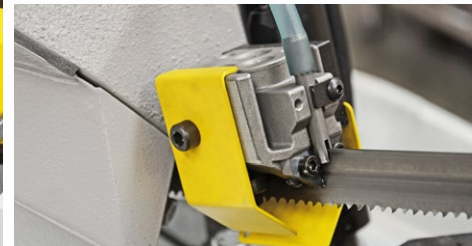
The saw blade guidance is enabled by ground hard metal elements of cemented carbide, always providing the greatest accuracy of the cut
