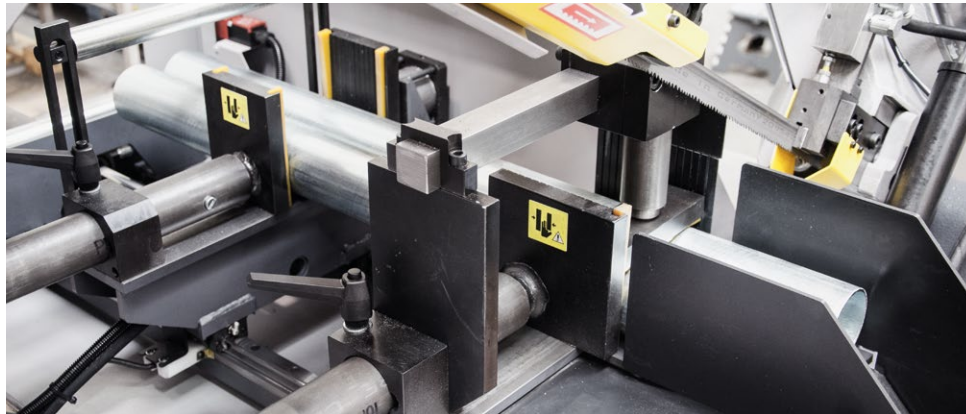
Robust feeding vice with hydraulically jaw
